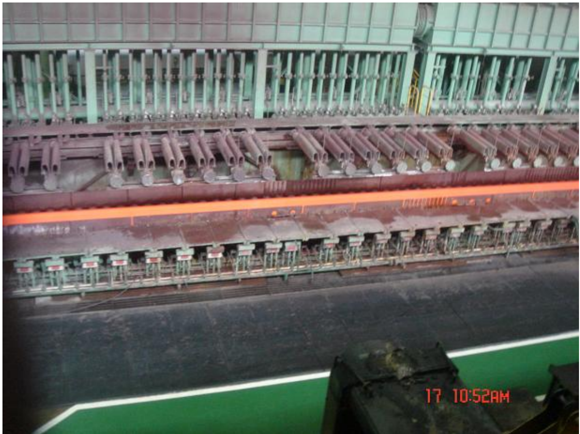
Production of Long thin Sheets ( Final Rolling)
