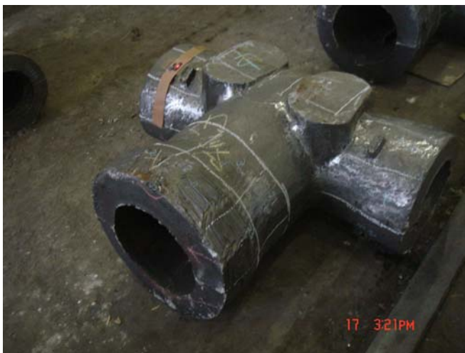
Heavy Casting Ready for Radiograph using LINAC
