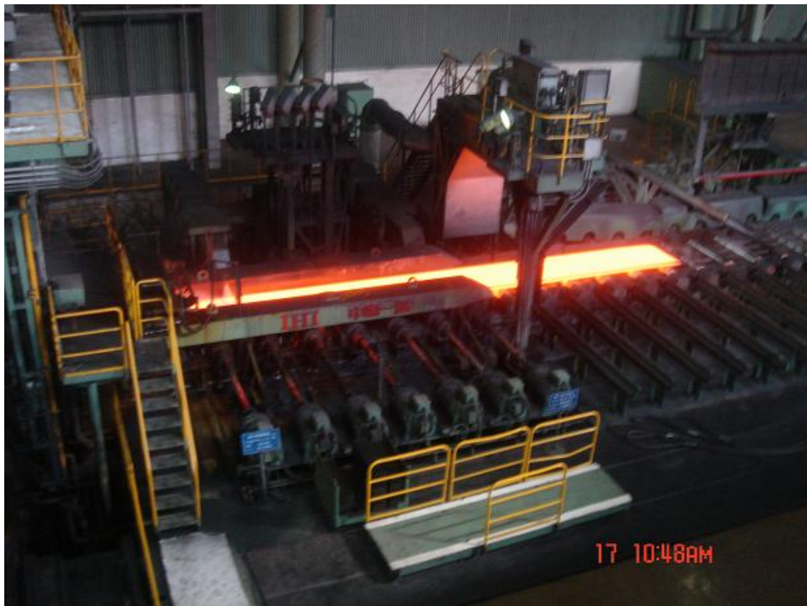
Picture above: Reduction of thickness by Hot Rolling (Rough Rolling)
